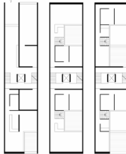
Fig. 8: 35 ha Area 7.5 m Housing Typology, Ground Floor to Third Floor, Source: TU Berlin
