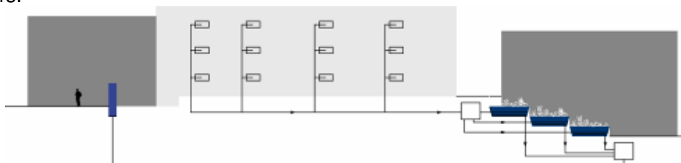
Fig. 10: Grey water reuse in decentralized constructed wetlands, Source: inter 3, Berlin
