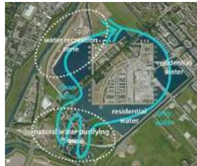
Simplified scheme closed water system
