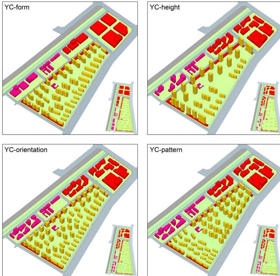
*Figure 3 The four experimental models based on consideration of the following parameters: form (upper left) average building height (upper right), orientation (lower left) and community pattern (lower right).*
