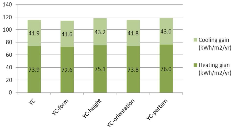
Figure 8 The comparison of annual energy demands between the prototype and experimental models
