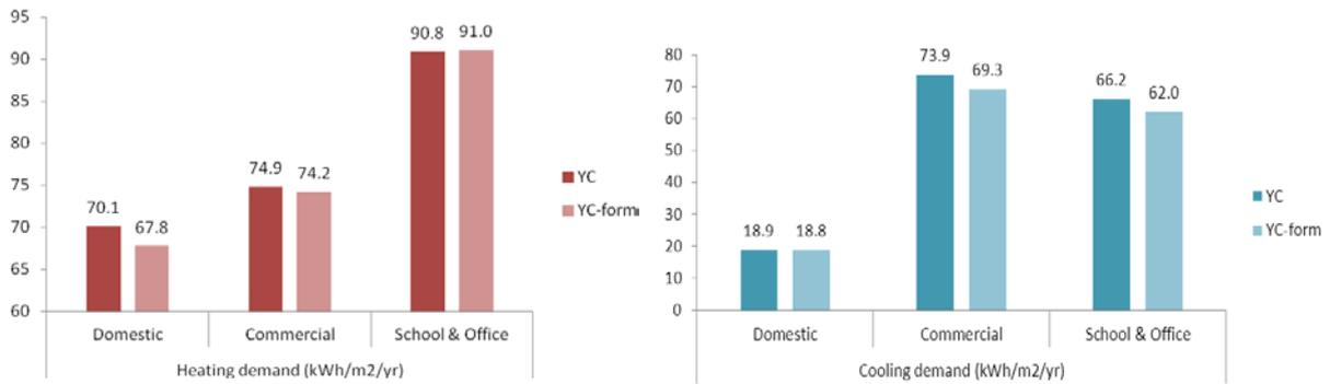
Figure 4 Comparison of energy demands between the prototype and the experimental models with different building forms.
