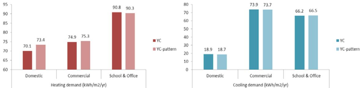
Figure 7 Comparison of energy demands between the prototype and the experimental models with different community patterns.
