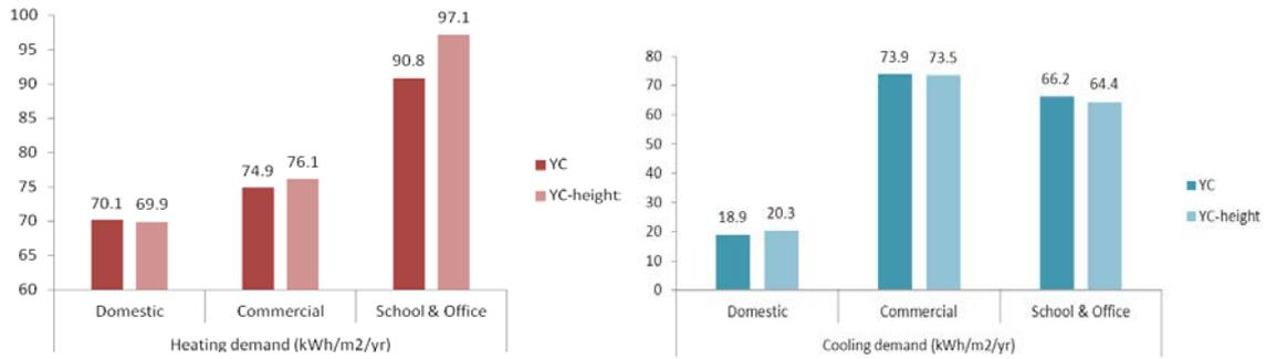
Figure 5 Comparison of energy demands between the prototype and the experimental models with different average building height.
