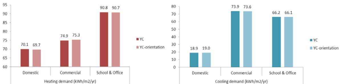
Figure 6 Comparison of energy demands between the prototype and the experimental models with different orientations of buildings.
