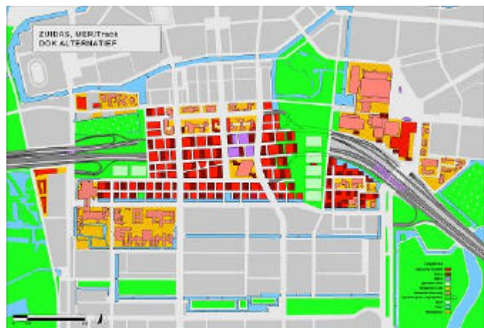
Figure 3: Zuidas master plan 2001: the bundle of infrastructure is covered, creating the conditions for a new area of multiple intensive land use
