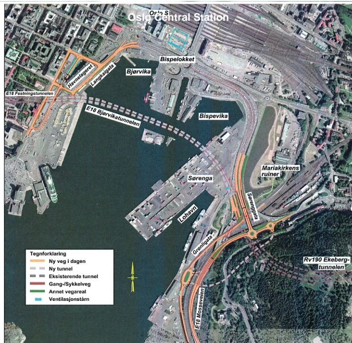
Bjorvika today. The double dotted line indicates the new suspended tunnel that is a precondition for development of the area (source: PBE, Oslo).
