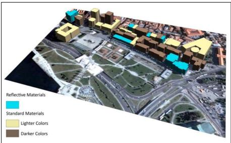
Figure 4. Building height and surface cover materials (Drawing by the author on the image from Google Earth)
