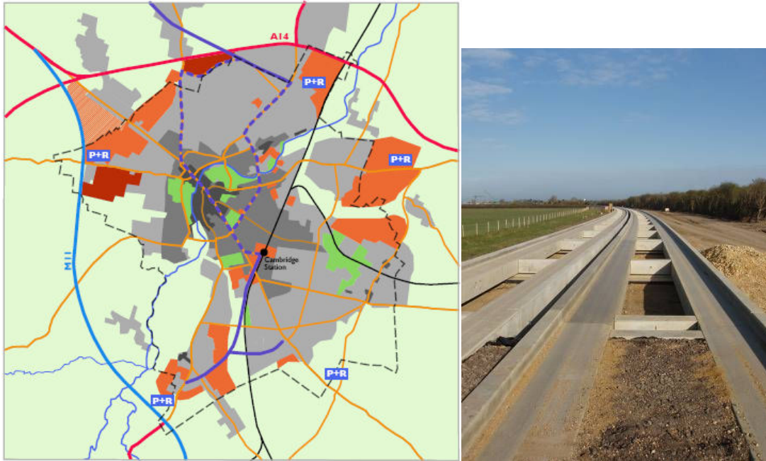
Figure 5 Cambridge Guided Bus route under construction (NB the dark blue lines show the guideways within the Cambridge part of the route. The dotted blue lines are the on road sections)
