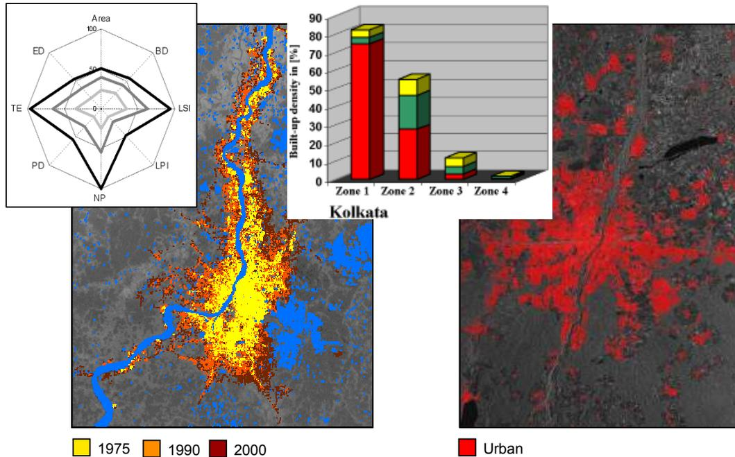
Fig. 1: Time series analysis of Landsat data for Kolkata, India (left), and urban footprint of Munich, Germany, derived from TerraSAR-X data (right). The spider diagram for Kolkata shows the development of different landscape metrics from 1975 – 2000.
