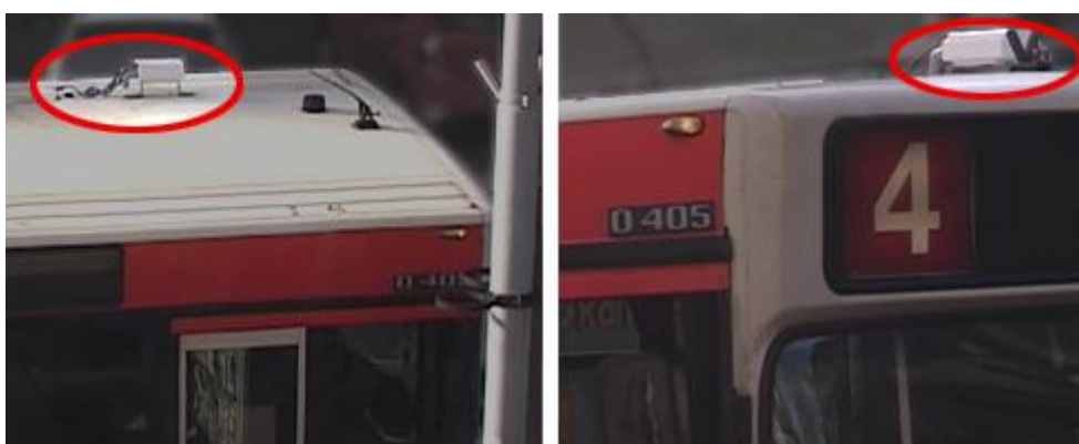
Figure 2 - EcoBus instrument mounted onto public transportation vehicles (Source: Bielsa, 2012)
