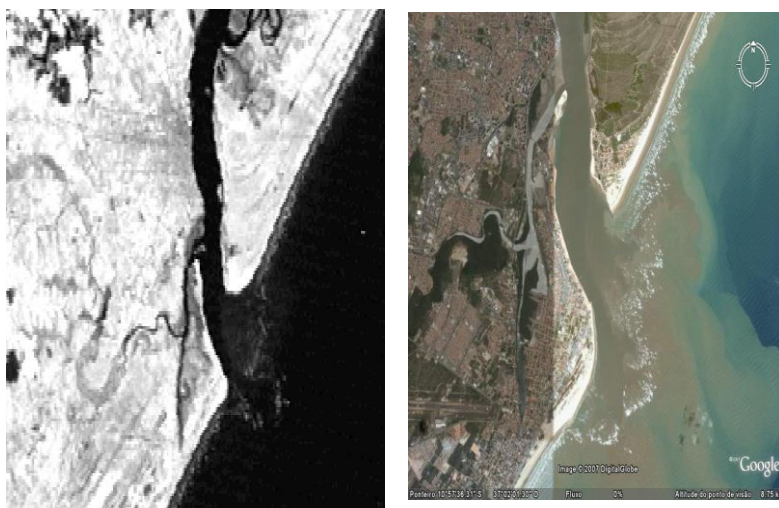
Figure 5: Comparative image of the estuary of Rio Sergipe. To observe the occurred changes in the morphology of the mouth of a river. Photos of the years of 1979 (satellite Landsat 2) and 2004 (Google Earth), respectively.
