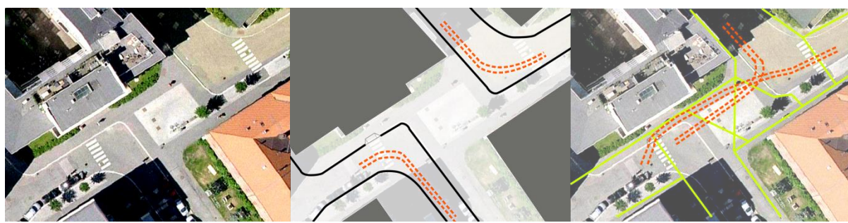
Figure 7 Aerial view of the plaza (left), drawing of traffic intention, traffic and pedestrian conflicts (right – car traffic in orange, pedestrian in yellow-green).
