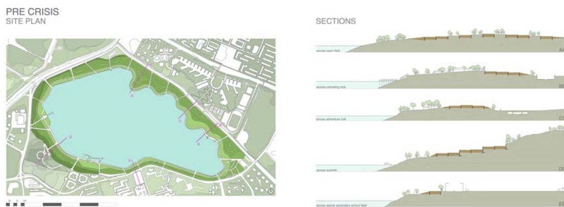
Figure 23: Stockpiling of Topsoil around Bedok Reservoir
