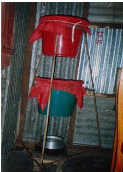
Photograph 07 (a): Bucket Filter.
